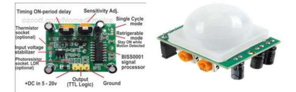
When a human body or any animal passes by, then it intercepts the first slot of the PIR sensor. This causes a positive differential change between the two bisects. When a human body leaves the sensing area, the sensor generates a negative differential change between the two bisects. The infrared sensor itself is housed in a hermetically sealed metal to improve humidity/temperature/noise/immunity. There is a window which is made of typically coated silicon material to protect the sensing element.
